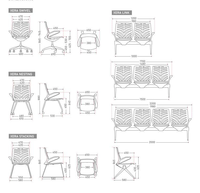
Remark: All dimensions shown are in mm. Tolerance is  $\pm 5$  mm.
